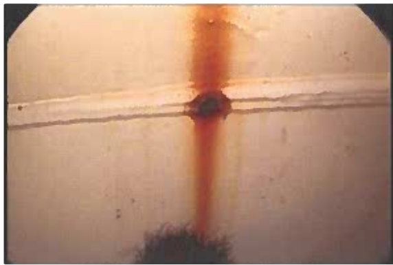
6:52 Brushed corrosion cell
